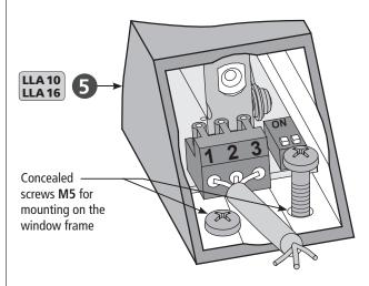
■ Secure fasteners against loosening; e.g. by applying removable thread-locking compound such as "Loctite".
