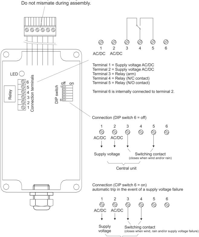
For assembly, remove plug connection from the cover.
