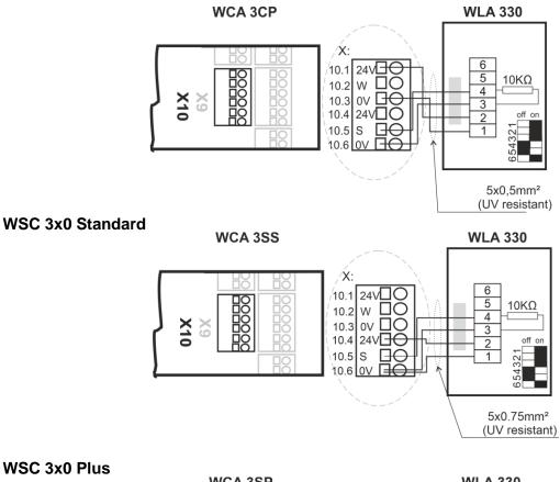
WCA 3SP WLA 330 ⁄X:  $\begin{array}{c|c} & & & \\ 10.1 & 24 \\ \hline 10.2 & W & \Box \\ 10.2 & W & \Box \\ 10.3 & 0 \\ 10.4 & 24 \\ \hline 10.5 & S & \Box \\ 10.6 & 0 \\ \hline \end{array}$ 6 5 4 3 2 1 10KΩ X10 S S off on 654 5x0.75mm<sup>2</sup> (UV resistant)
