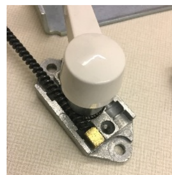
End Stop Preventing Inner Cable Coming Out of The Operating Handle Gearbox
