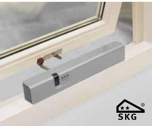
The AXA Remote 2.0 features an anti-trap system that interrupts the closing movement. If there is a risk of something becoming trapped between the window and the framework, the AXA Remote 2.0 will open.
